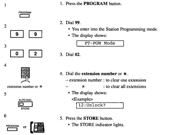
6. Press the **PROGRAM** button or lift the **handset** to exit from the Station Programming mode.
