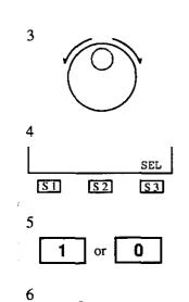
Rotate the Jog Dial until "Night On/Off" (for KX-T7436) or "Night Mode" (for KX-T7433) is at the arrow.
